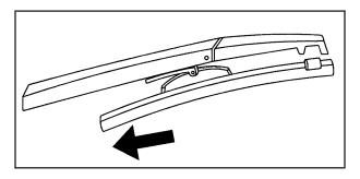
4. Remove clip (A), shown in step 3, and slide it into the claw of the wiper blade assembly.
